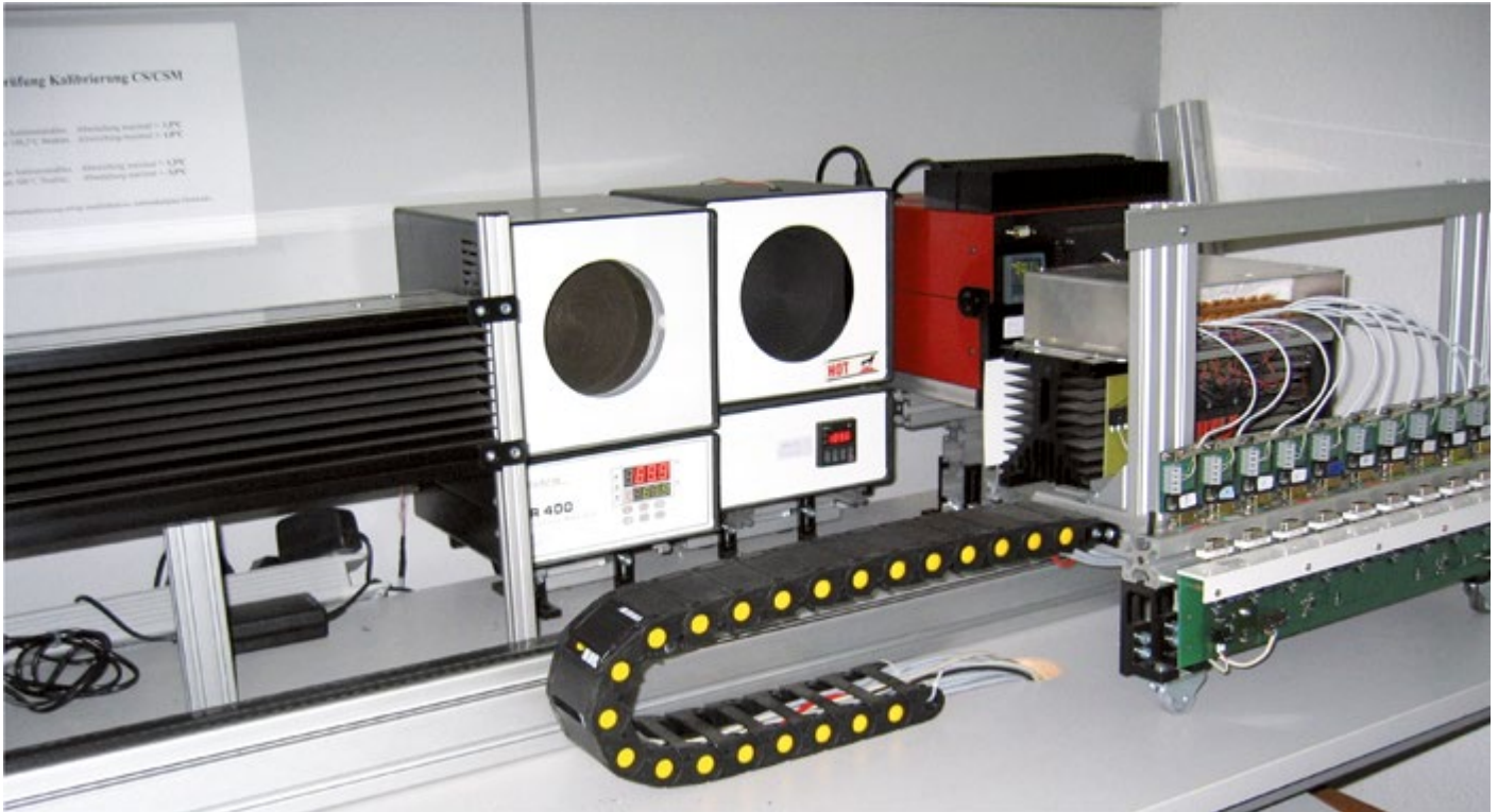
Automated calibration stations at Optris GmbH
