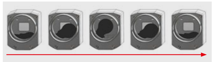
For offset compensation the whole field of view of an infrared sensor array is closed by a linear motor for a short time
